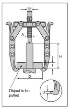
The reaching range of the claws can be expanded by shifting one hole type to two or three holes types. The steel ball installed in the adaptor significantly reduces friction.
