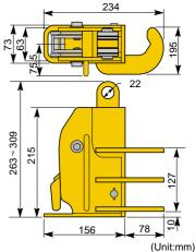
Equipped with Remote control and releasing mechanisms
