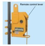
When the rope supplied with the clamp is connected to the remote control lever, the clamp can be easily detached from the work piece by pulling the remote control rope to lock the clamp into the open position.
