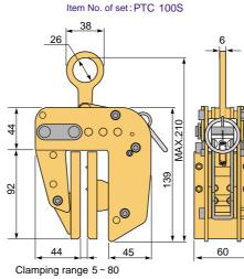
Optimal for lifting and installation of molded frames and wooden panels. Siding boards, decoration panels for outer walls, heatresistant external walls material, wooden panels. Do not use these clamps for ALC, extrusion forming boards.
