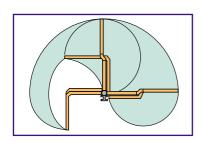
As the central joint of the arm can be turned as in the above figure, you can secure and effective use of a wide range of working area. (on the assumption that there is no obstacle around)
