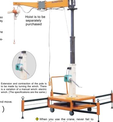
When you use the crane, never fail to extend the legs of the outriggers to the four different directions so as to provide stability.
