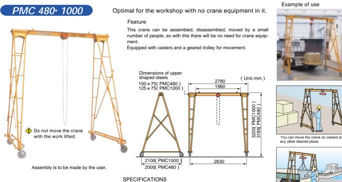
Rated capacity Lifting height Weight Item No. Remarks (kg) (m) (kg) PMC 480 480 3 320 PMC 1000 1,000 3 360
