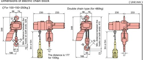
The length of power cord for the chain block is 5m. The length of the press button cord is 3 or 5m (same as lifting height).
