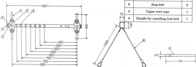
When lifting a long work piece, use this balance for stable lifting and handling.
