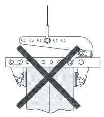
4. Ensure that the pads have securely clamped the work before the lifting operation.
