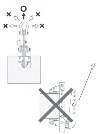
When you lift the work at two points, use the simple balance so that the work is vertically lifted at two points.
