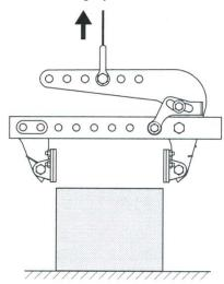
5. If you lift the work away from its central gravity point, the gripping position of the clamp threatens to slide, which may cause an incident. So, never do that.
