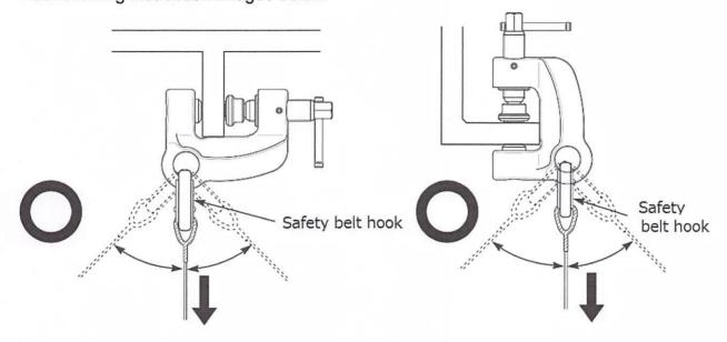
As following instruction images, the safety belt hook or rope must not be touched with the main body or screw handle. Also please do not let the clamp get rotated by the impact in any wrong way of using.
