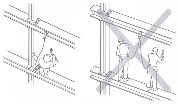
This safety belt clamp must not be used for any operations of pulling or lifting.
