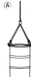
Using two clamps (This is safe when lifting a heavy drum, containing, for example, iron powder.)
