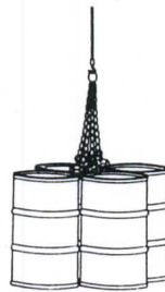
Lifting four drums with four clamps (in this case, the drums are lifted vertically.)
