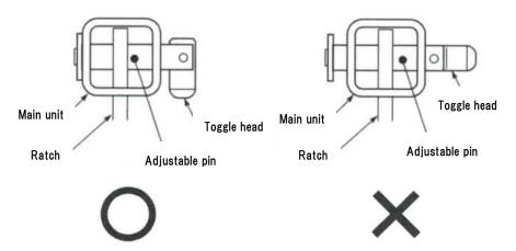
2. Adjust the position of the shackle according to the central gravity points.
