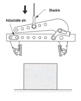
3. When the release lever is raised by pressing down the arm with your hand, you are now in a position to lift the work.
