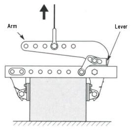
(4) After carrying the work to the destination, lower the clamp till the wire rope is fully loosened.
