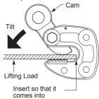
Insert so that it comes into contact with the deepest section.
