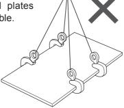
7 Vertical lifting is not possible with this clamp. For vertical lifting, be sure to use vertical lifting clamps or screw cam clamps.
