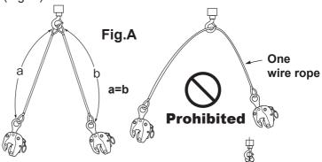
10. When lifting at 2 points, keep the lifting angle within 60°. (Fig. B)
