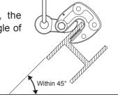
5 The clamps can also be used for temporary turning over H steel, etc.
