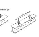
4 If the load is lifted at an angle, the clamp should be inclined at an angle of up to  $45^{\circ}$ .
