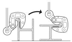
6 Even with 2 or 4 points lifting, horizontal lifting of steel plates and flat plates is not possible.
